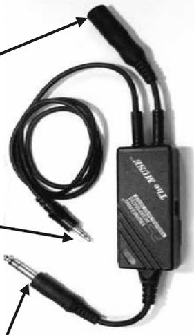
entertainment device. When the entertainment device is not playing, the unit is in the "sleep mode". This "sleep" mode requires an incredibly small amount of current (17µA). The instant that *The Muse*® detects a signal on the music input line, it turns itself on. When the signal goes away, it turns itself back into the "sleep" mode. This is completely automatic, you'll never have to turn the unit off, or unplug any cables.
