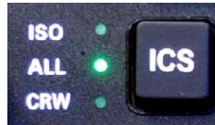
**ISO:** The pilot is isolated from the intercom and is connected only to the aircraft radio system.
