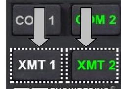
Select either of the com XMT buttons to exit the **split** mode. It is not possible to have the pilot on COM 2 and copilot on COM 1 in **split** mode.
