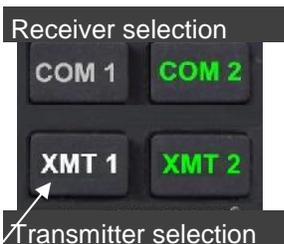
In normal (not Split) modes, the PMA8000G gives priority to the pilot's radio Push-To-Talk (PTT). If the copilot is transmitting, and the pilot presses his PTT, the pilot's microphone will be heard over the selected com transmitter.
