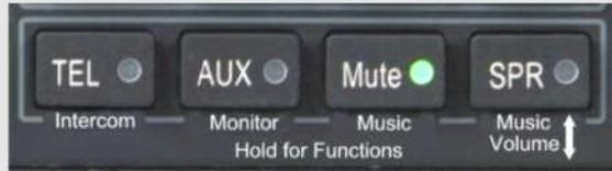
dio when it is active. For example, if COM 1 is selected to transmit to ATC, but COM 2 is receiving weather information; the ATC will mute the audio from the weather while ATC is transmitting. In Monitor mode, the RCV COM indicator will blink every few seconds as a status indication. Monitor mode is set off when the unit is turned off.
