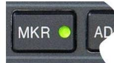
Holding the MKR button for one second also activates marker test, labeled "T/M" and illuminates all three lamps (internal and external) are working. Releasing the button returns to the last sensitivity.
