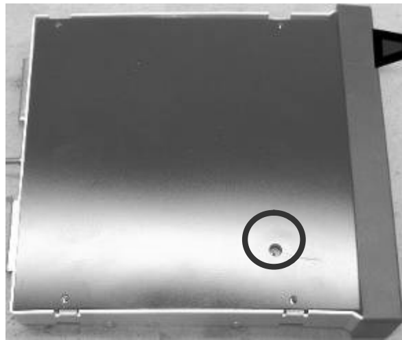
Figure 2-5 – Unswitched 3 Audio Level (bottom cover removed)
