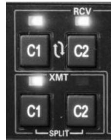
To select a VHF COM radio to listen only, push the C1 or C2 button in the RCV (Receive) section.
