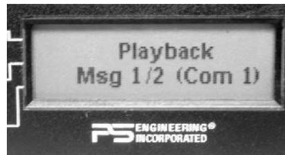
The screen displays a status message to indicate that playback is in progress. The playback will stop whenever there is more incoming selected com audio, and the message can be replayed from the beginning by pressing the selected Com Receive button again for 1 second.
