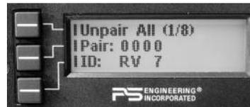
There are three Bluetooth functions that can be changed in the user setup screen, Unpair All, Pair PIN code, and device ID.
