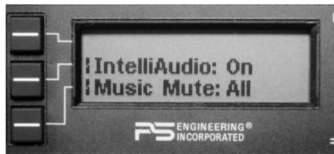
ity in a very logical manner. Press the line select key to select a specific item on each menu. Items are toggled on and off by pressing the line select key as well.
