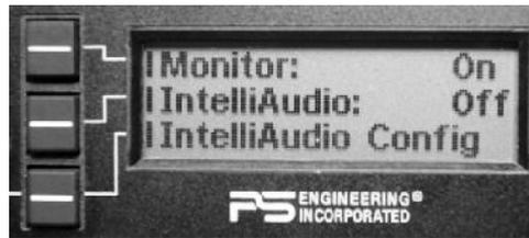
To toggle the Monitor mode on and off, Press and hold **IntelliAudio MONITOR**
