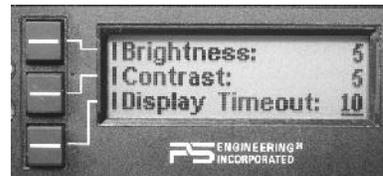
There are two modes: LCD Brightness & LCD Contrast.
