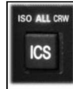
**ISO** (Pilot Isolate): The pilot is isolated from the intercom and is connected only to the aircraft radio system. He will hear the aircraft radio reception (and sidetone during radio transmissions). Copilot will hear passengers' intercom and Music, while passengers will hear copilot intercom and Music. Neither will hear aircraft radio receptions or pilot transmissions. The pilot can hear music if desired.
