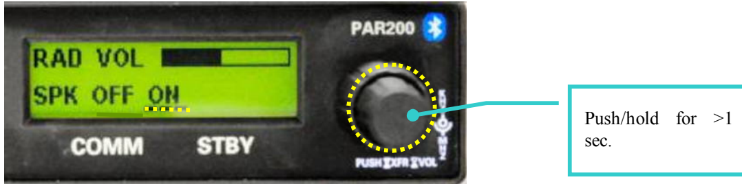
Figure 3-4 Cockpit Speaker Control
