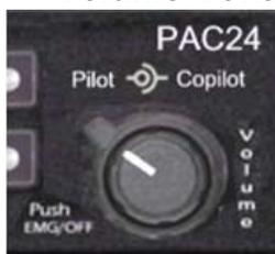
The volume control is a concentric knob. The inner knob adjusts the loudness of the intercom for the pilot (in single panel installation) and the outer knob controls copilot and passenger volume. It has no effect on selected radio levels or music input levels.
