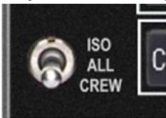
**CREW:** Pilot copilot and passengers are connected on one intercom channel and have access to the selected aircraft radios. They may also listen to Entertainment.
