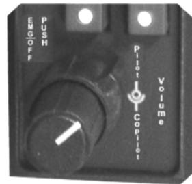
In dual installation, the inner knob controls the main volume (the person connected to the audio panel) and the outer knob controls the passengers.
