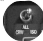
In a single panel installation without expansion, the passengers will also hear what the copilot hears
