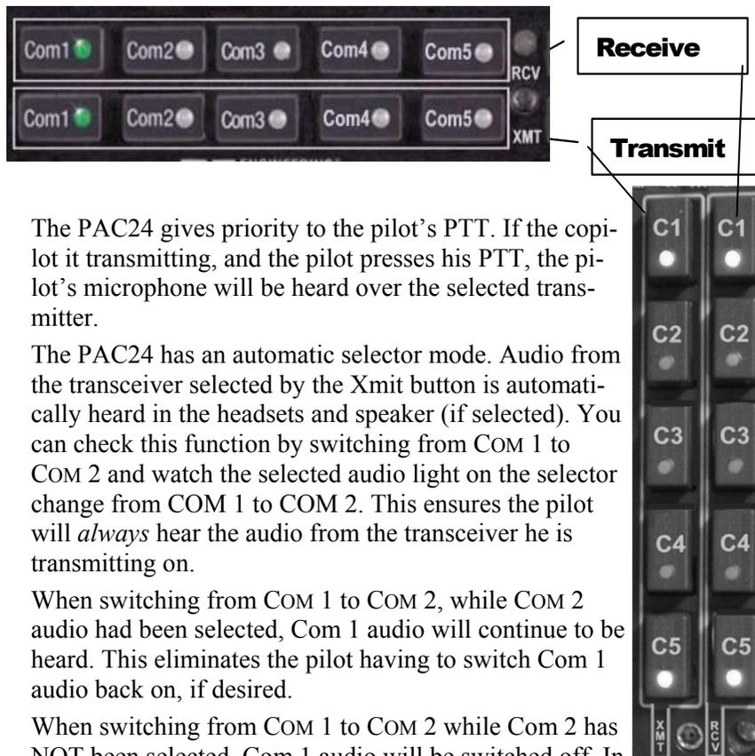
The PAC24 gives priority to the pilot's PTT. If the copilot is transmitting, and the pilot presses his PTT, the pilot's microphone will be heard over the selected transmitter.
