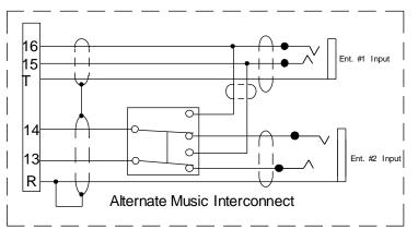
**NOTE**: Use the <u>low level</u> output of any additional entertainment device to connect to the audio panel. Maximum signal level is **2 VAC** p-p. **DO NOT** use a speaker-level output, this will cause internal damage in the audio panel.
